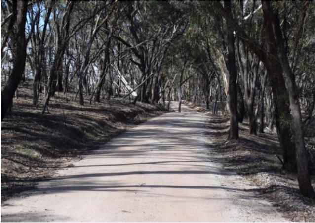
**Figure 7.9 Narrow access on Mount Kerang Road identified as providing poor line-of-sight, no passing opportunities for large vehicles and caravans, and difficulty to reverse due to narrowness and bends in road**
