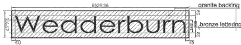
Curved Bronze Strip - Frame and Fixing Detail (Typical Section) Scale 1:20
